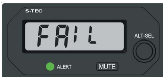
Fig. 4-1. Altitude Selector / Alerter Fail Indication
