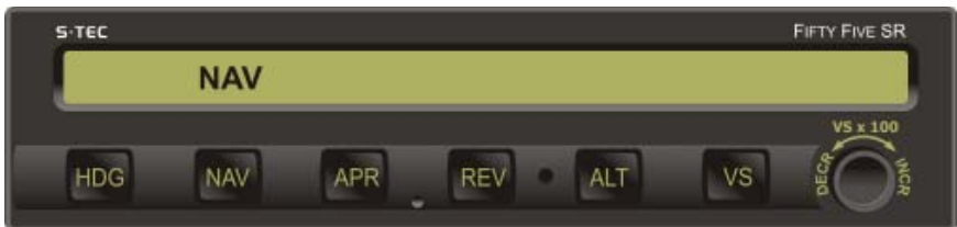
Fig. 3-2. AP Display, NAV Mode Engaged
