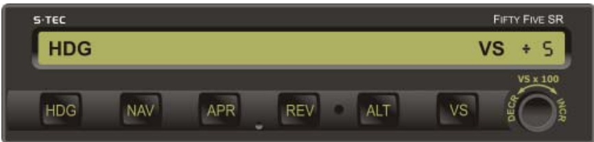
Fig. 3-8. AP Display, HDG and VS Modes Engaged
