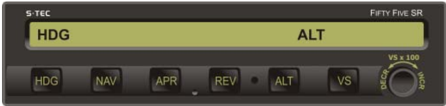
Fig. 3-7. AP Display, HDG and ALT HOLD Modes Engaged
