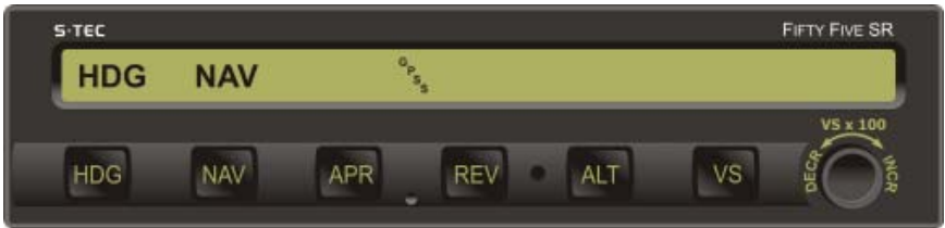
Fig. 3-6. AP Display, HDG Mode Engaged, NAV GPSS Mode Armed
