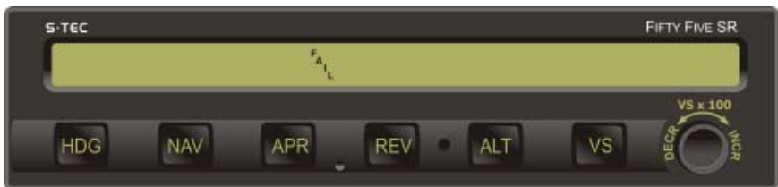
Fig. 2-4. AP Display, Programmer/Computer Failure
