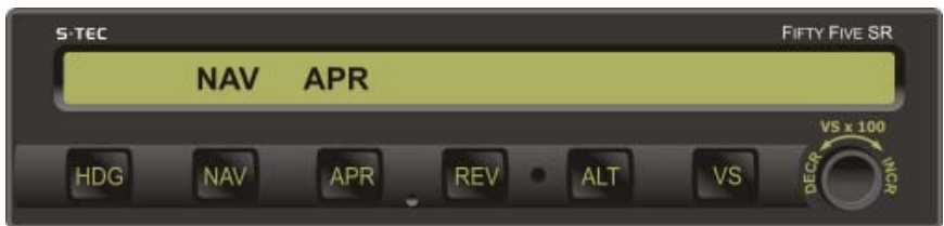
Fig. 3-22. AP Display, NAV APR Mode Engaged, Track LOC Front Course Inbound
