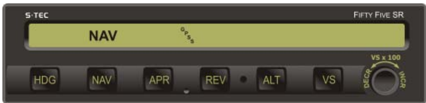
Fig. 3-5. AP Display, NAV GPSS Mode Engaged
