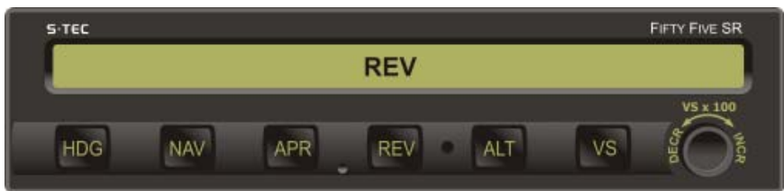
Fig. 3-11. AP Display, REV Mode Engaged, Track LOC Back Course Inbound
