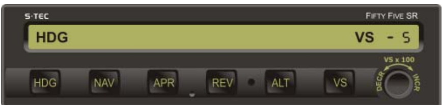
Fig. 2-9. AP Display, HDG and VS Modes Engaged, 500 FPM Descending (Pre-Flight)
