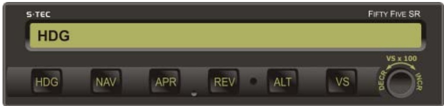
Fig. 3-1. AP Display, HDG Mode Engaged
