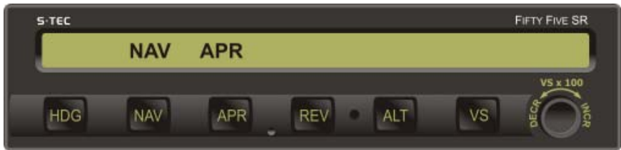
Fig. 3-17. AP Display, NAV APR Mode Engaged, Track LOC Front Course Inbound
