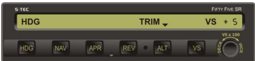
b. TRIM DN in Progress
