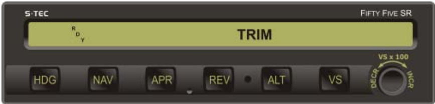
Fig. 3-10. AP Display, Manual Electric Trim in Progress
