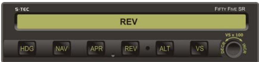
Fig. 3-15. AP Display, REV Mode Engaged, Track LOC Back Course Inbound
