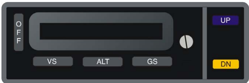
Fig. 2-2. AP Display, All Annunciations Extinguished
