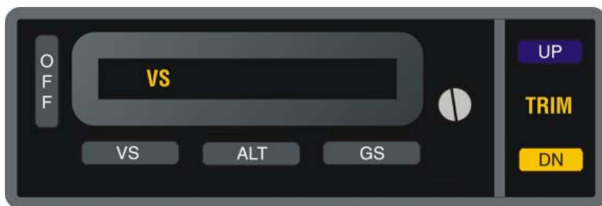
Fig. 2-5. AP Display, VS Mode Engaged, TRIM Required
