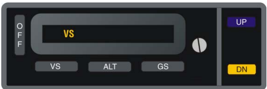
Fig. 2-3. AP Display, VS Mode Engaged
